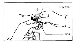
To remove the bit, push the sleeve up toward the "FREE" side and turn the sleeve counterclockwise while holding the ring with your other hand.
